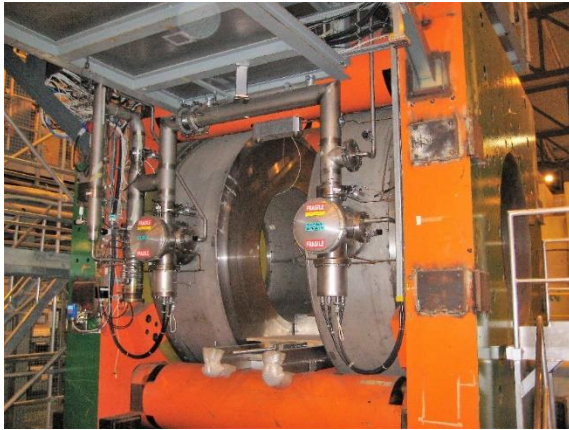
Figure 37: Beam line test facilities in use in EHN1: the 3-T CMS-M1 magnet (left), and the 1.9-T Morpurgo dipole (right).
