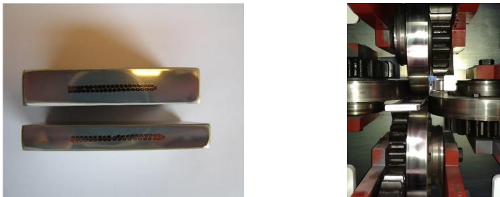
Figure 36: Cold work of an Al-0.1wt%Ni stabilized conductor with an Atlas-BT cross section (CLICdp studies).
